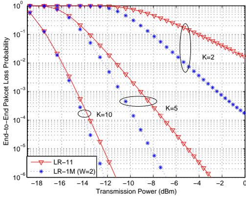
**Figure 6.** ETE packet loss rate for LR-11 and LR-1M schemes as a function of transmission power in an equidistant line network with the constraint on the maximum number of transmissions  $K = \{2, 5, 10\}$  in truncated ARQ
