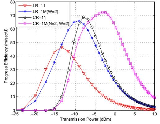
**Figure 4.** Progress efficiency for all schemes in consideration as a function of transmission power in an equidistant line network with  $M = 100$  and source-destination distance  $d = 1000m$
