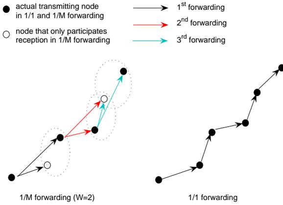
**Figure 1.** Comparison of the basic operation of 1/M forwarding policy and 1/1 policy
