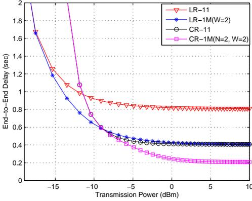
**Figure 3.** ETE delay for all schemes in consideration as a function of transmission power in an equidistant line network with  $M = 100$  and source-destination distance  $d = 1000m$
