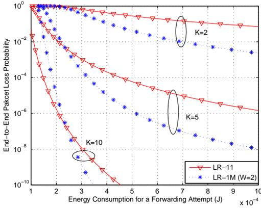
**Figure 7.** ETE packet loss rate for LR-11 and LR-1M schemes as a function of energy consumption for a forwarding attempt in an equidistant line network with the constraint on the maximum number of transmissions  $K = \{2, 5, 10\}$  in truncated ARQ
