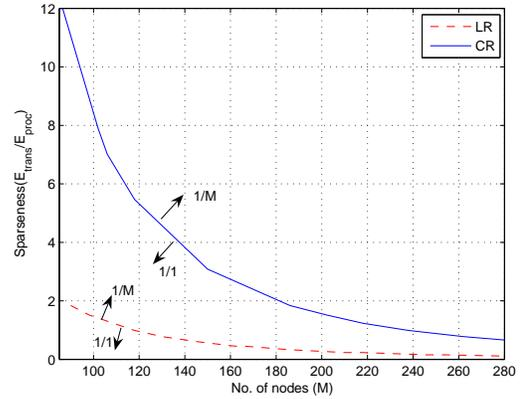
**Figure 5.** Minimum required sparseness  $E_{trans}/E_{proc}$  for 1/M policy to outperform 1/1 policy in both LR and CR strategies in an equidistant line network with  $M$  relays
